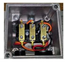
The terminal box of a 3-phase asynchronous motor - star connection/Y
